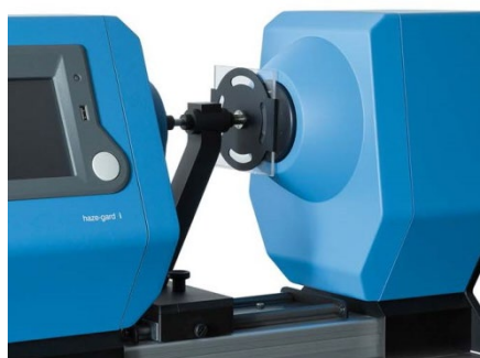
The measurement of haze is used to determine abrasion resistance of transparent materials. The haze-gard i Abrasion Holder facilitates positioning of the abraded area in the measurement beam.
